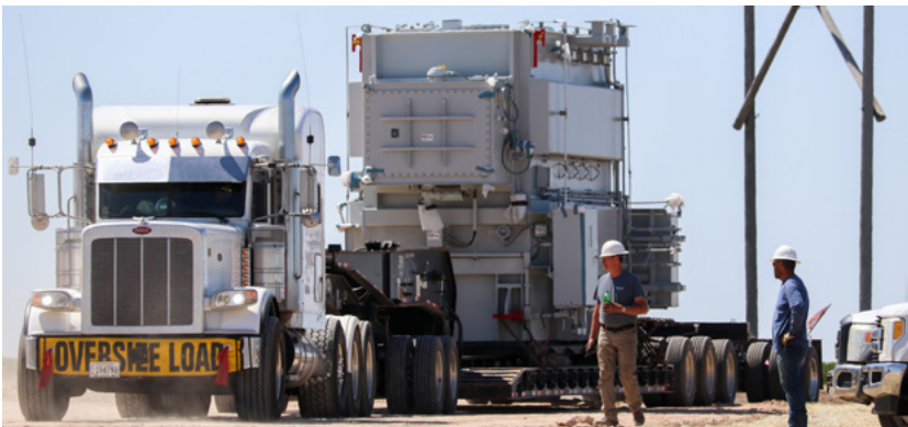
Crews move a transformer to the Butter and Egg Substation.
